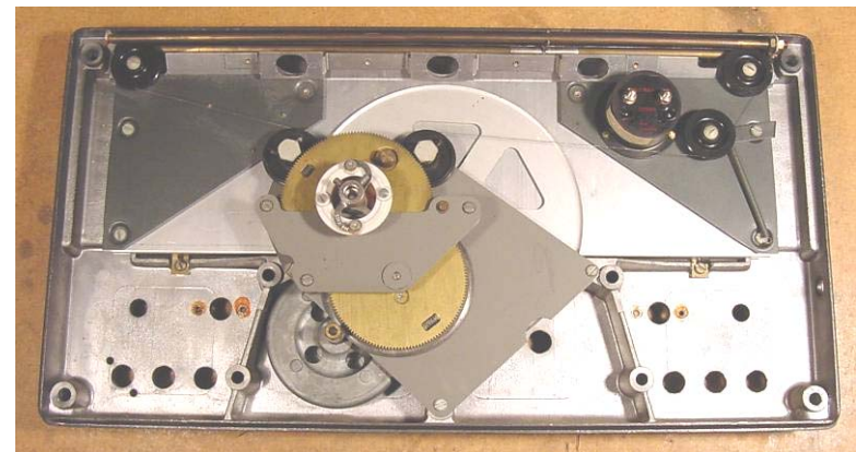
Above: Photos of the drive train from an S.680X – again, almost identical to the S.750 (but with a smart paint finish on the gearbox sides).
