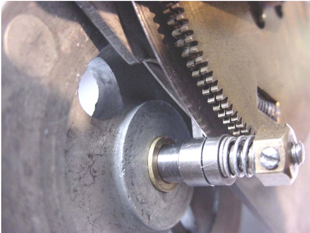
Above: 'peek-a-boo' view of the dial mechanism fitted into my recently powder-coated black crackle S.750 case (also shown on the photo on previous page). Below: close-up of the pinch wheel and friction plate. Note the brass insert in the flywheel.
